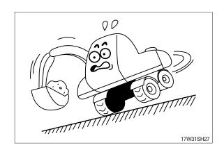
Avoid parking and stopping on a slope. Lower the bucket to the ground and block the tires when parking.
